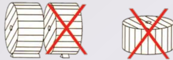
Do not lay drums flat on their sides, use proper stops to prevent drums rolling.
